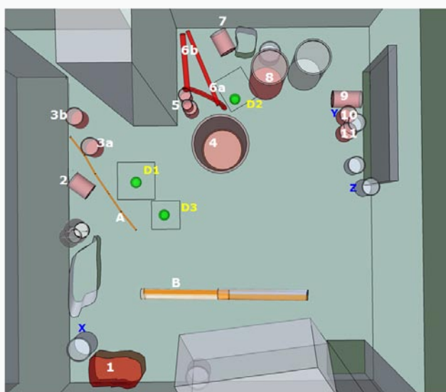
Figure 5: Final triangulated results from all three deployments showing source locations
