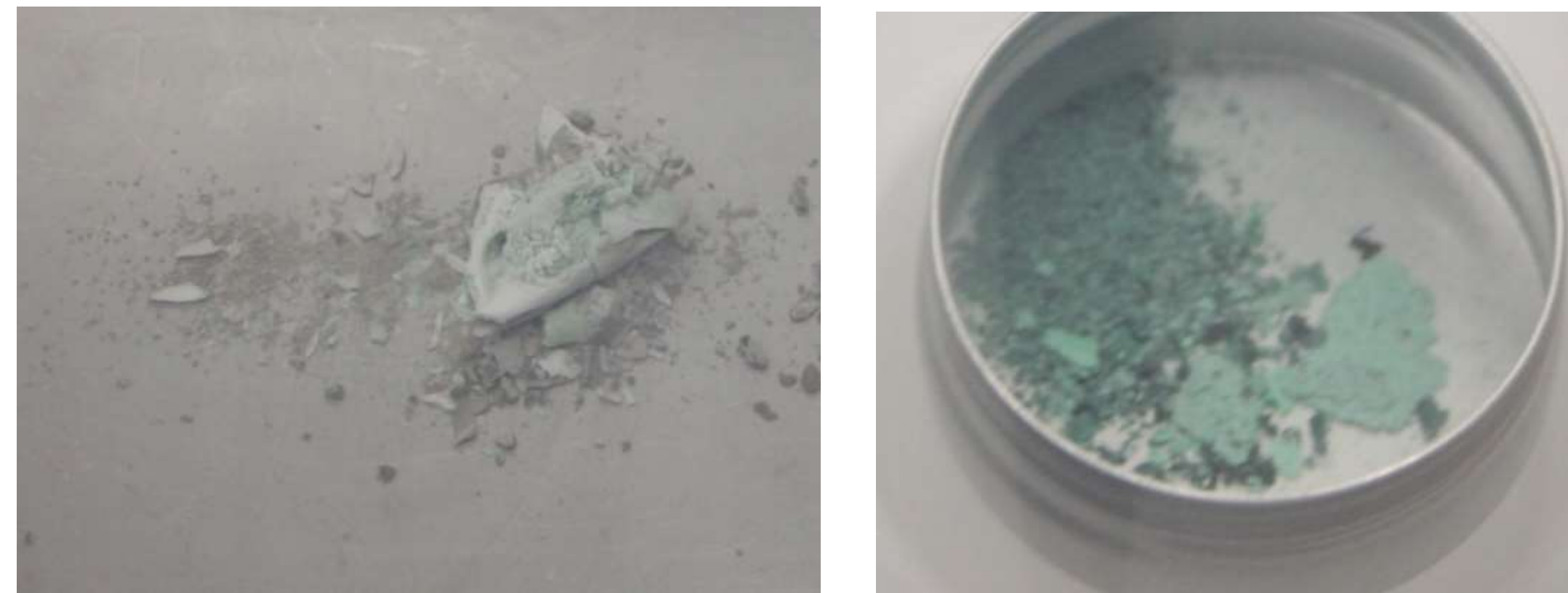
The reaction product produced from UF_6 reaction with ammonia at 200°C (Left) and 300°C (right)
