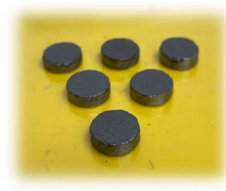
FIG2: batch of UN samples fabricated via SPS, samples are 10 mm in diameter.
