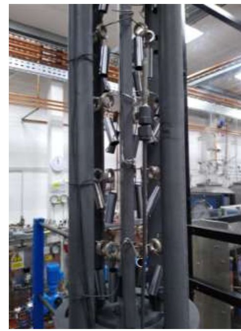
Figure 1: Cr-coated fuel tube specimens suspended within the autoclave space awaiting lid placement.
