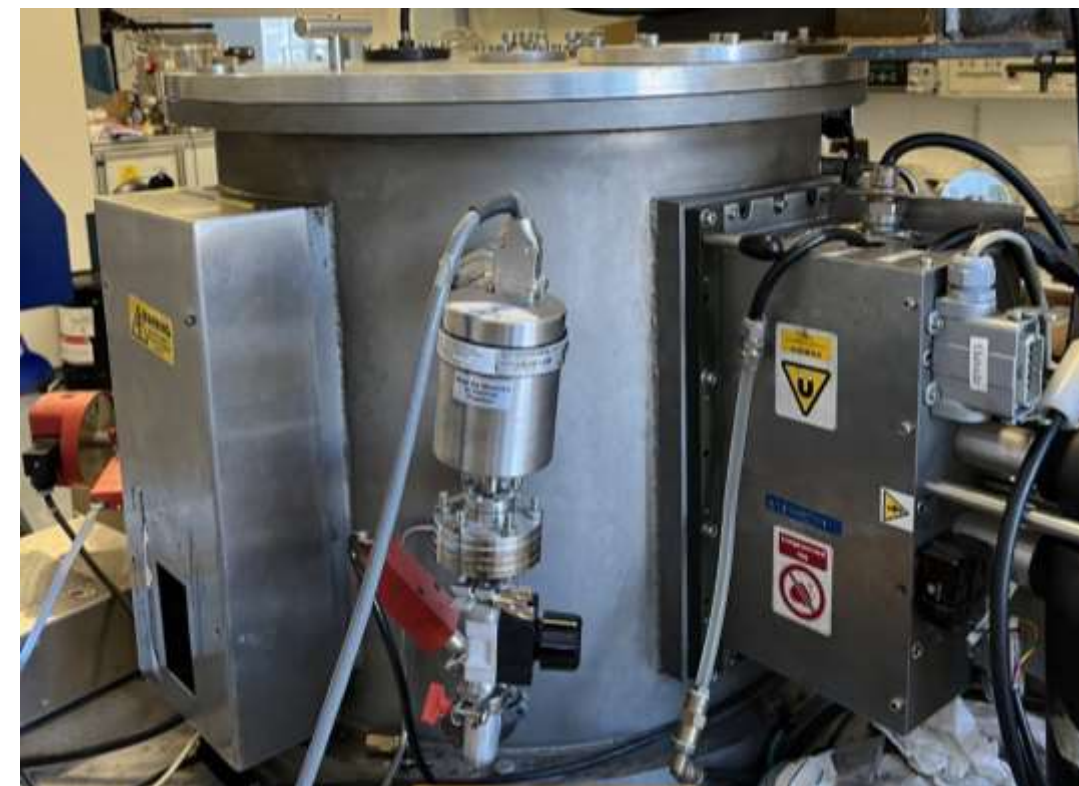
Coating deposited by magnetron sputtering using UDP450 chamber from Teer coatings
