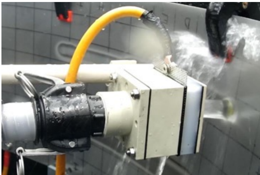
Prototype of the EASD jet system for cleaning vessel walls.
