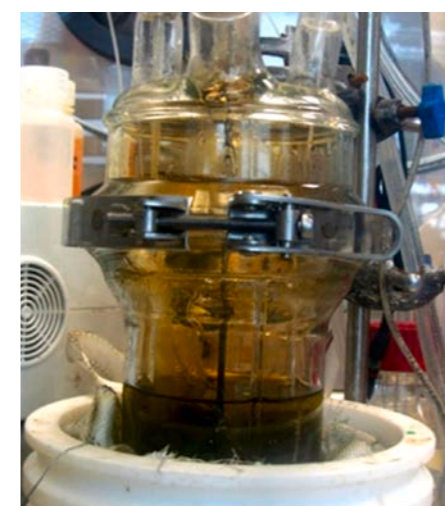
Mixed oxide fuel dissolution taking place in a glovebox. Taken from: R Taylor, G Mathers, A Banford, Progress in Nuclear Energy (2023) 164, 104837
