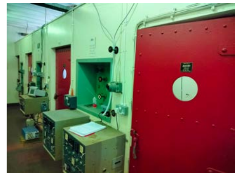
The joint coolant testing facility at University of Bristol, showing the cells containing high-temperature, high-pressure water and helium apparatus, heater controllers and monitoring instrumentation.
