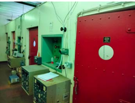
The joint coolant testing facility at University of Bristol, showing the cells containing high-temperature, high-pressure water and helium apparatus, heater controllers and monitoring instrumentation.
