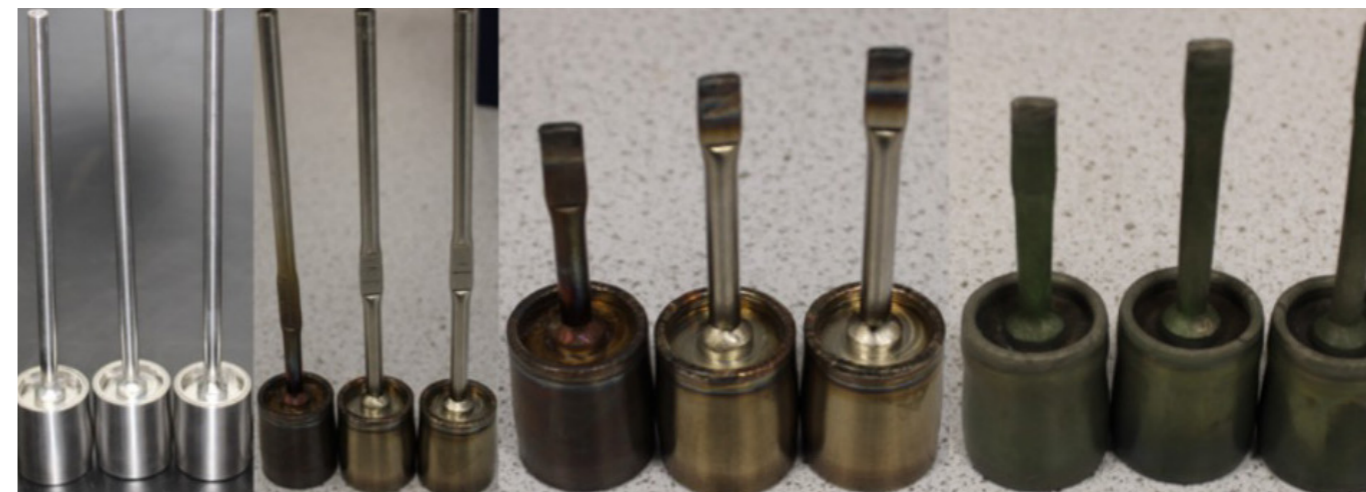
Graphite and glass HIP can at various processing stages: packing; bakeout; crimping; post HIP.
