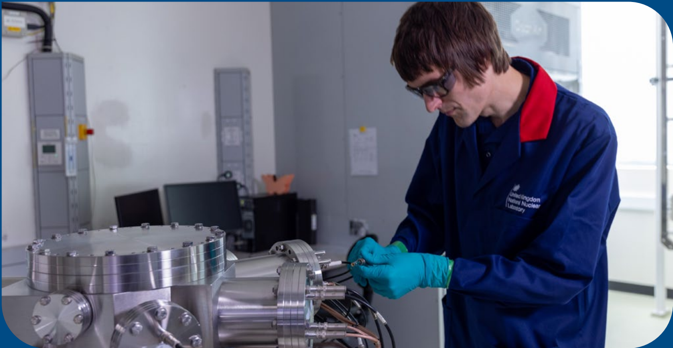
Setting up the mass spectrometer for material inspection at the Nuclear Materials Research Centre
